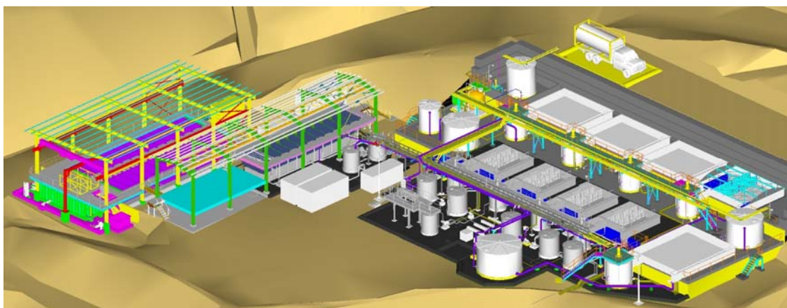
Figure 5: 3D design of EDP with new cell house and mixers/settlers (courtesy of NeuBau Pty Ltd).
