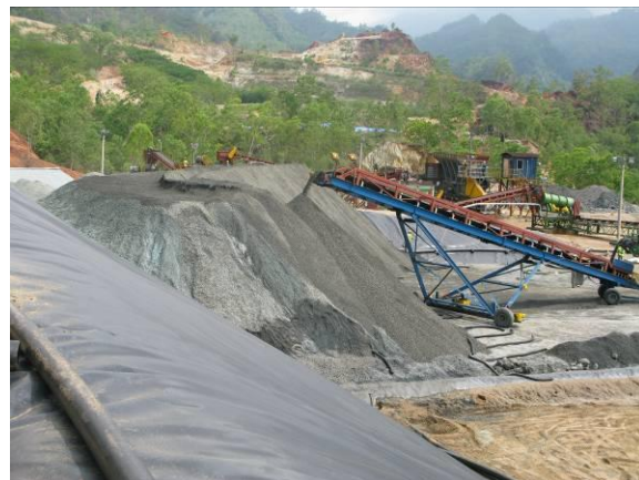
Ore stacking on demonstration heap, crusher in background
